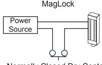
Normally Closed Dry Contact from intercom/relay
